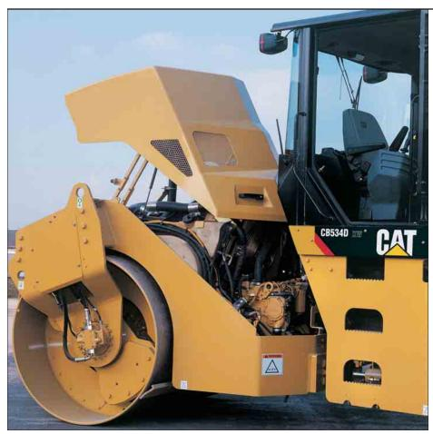
**Swing-open hood.** Large, swing-open hood on the machine provides easy access to routine maintenance points. The hood also provides access to the top of the engine.
