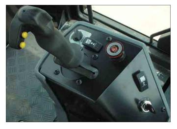
**Propel handle.** The multifunction ergonomic propel handle simplifies operation with the following controls: propel speed, vibe on/off, water spray on/off, horn and drum offset (optional).
