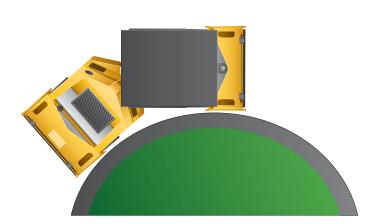
**Centered articulation.** The centered articulation with 50% of the machine length behind the pivot and 50% forward delivers evenly balanced weight front to rear. Drums track in the same path even in turns.
