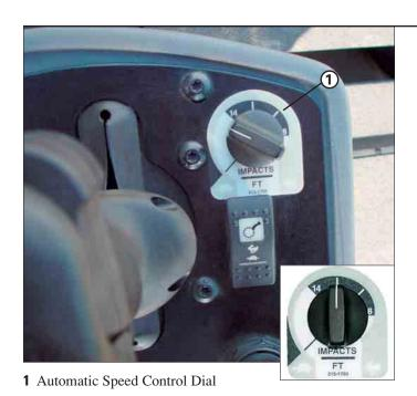
**ASC control.** Standard ASC control greatly simplifies operation by allowing the operator to preset machine speed or impact spacing.
